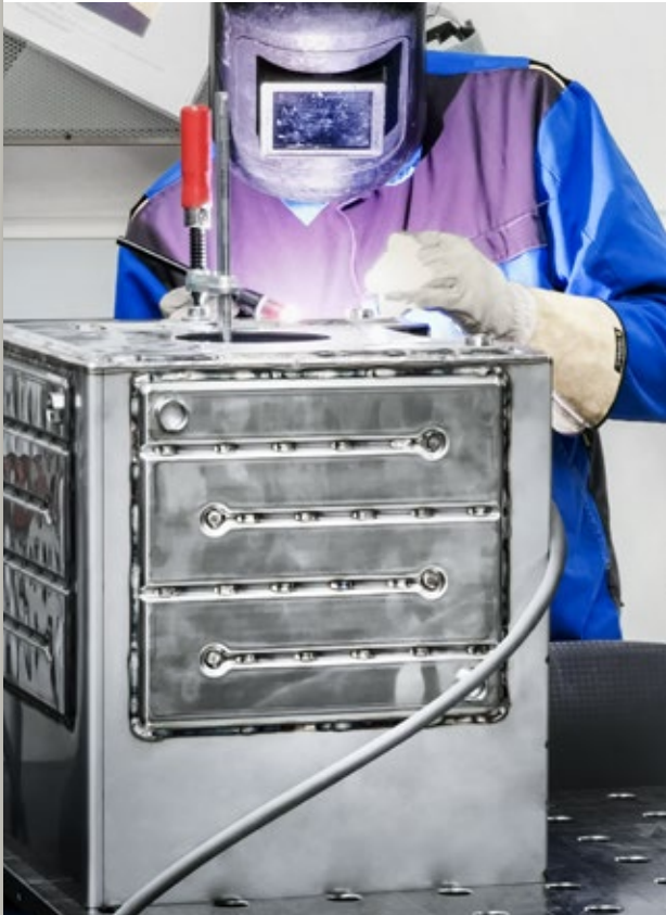
The heat exchangers are welded to the inside walls of the tank.
